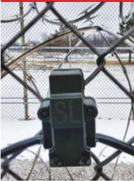
The SL-3 sensor installed on site. (Photo: RBtec)
